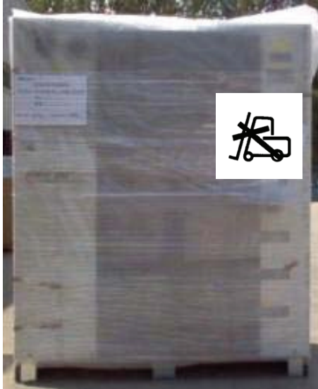
Figure 8-2 : Do not lift from the front unless strictly necessary
