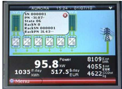
Figure 14-6: 50kW modules information
