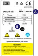
A) Inverter/battery model B) Main technical data
