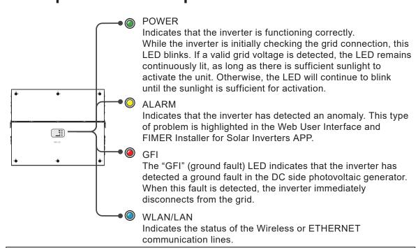
NOTE – The LEDs, in various multiple available combinations, can signal multiple conditions other than the original single condition; see the various descriptions explained in the "LEDs behaviour" paragraphs on this manual.
