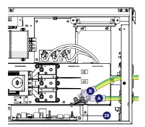
ATTENTION - Depending on the version of the AC panel installed on the inverter it will be necessary to use a different protection earth connection point in order to avoid mechanical stress due to cable bending: in
