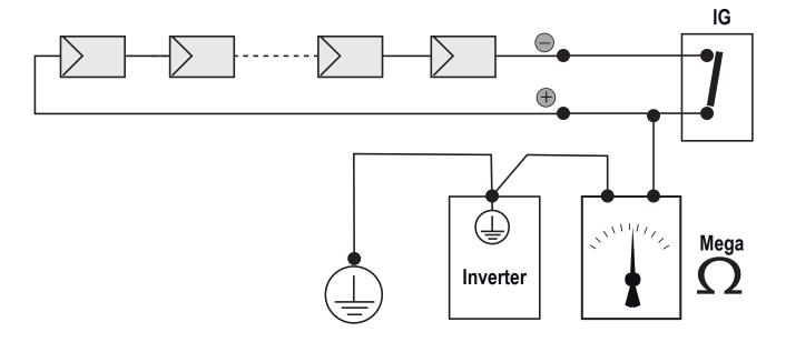
If the measured isolation resistance (Riso) is less than 75 kOhm, the inverter may not connect to the grid because of low isolation of the PV generator to ground.
