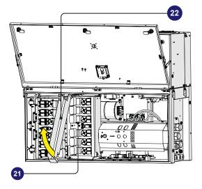
• Remove the three M5 screws from the DC surge arrester plate (21).
