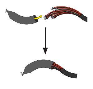
Pass the DC interface cables (33) into the wiring box using the dedicated opening for DC interface cables (30) as shown in the picture.
