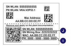
As an alternative of QR code scanning, claiming process can be executed by selecting manually the ESSIDs associated to the Wi-Fi networks generated by each inverter to commission and inserting Product key (I) when requested:
