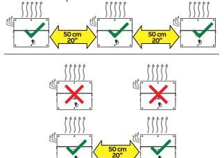
The installation of two inverters positioned back to back is also permitted on a structure which must
