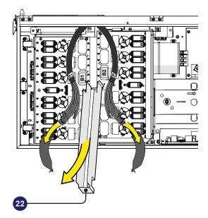
Connect all DC interface cables (33) to the related DC interface faston connectors (29) located in the DC surge arrester plate (21). The two cable group are marked with identification labels "B1" and "B2" that corresponds to the DSP board number label ("B1" and "B2").
