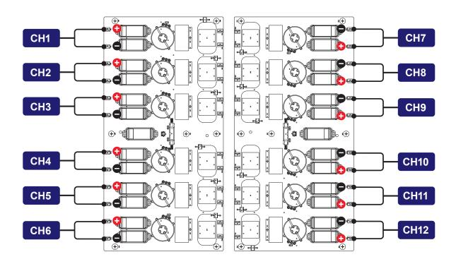
• For each input channel the measurement must be performed between: positive to ground, negative to ground, positive to negative.
