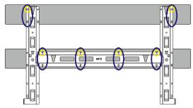
Frame mounting (2 supports) minimum fixing points
