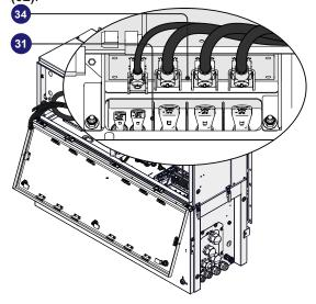
Remove the AC interface connections protective cover (58) (if present) by pressing the 2 sides latch.
