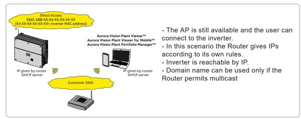
During the installation wizard, the installer will be asked to connect the inverter to a Wi-Fi router. By selecting connection to Wi-Fi router the inverter will turn on a second Wi-Fi radio channel in order to enable connection to the Wi-Fi router.
