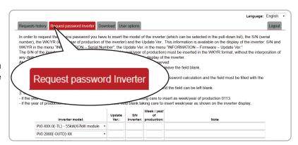
Choose the inverter model from the drop-down list and insert Serial Number and Week of Production of the inverter which were obtained previously (Stage 1).
