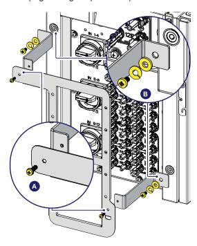
Connect the strings, starting from IN12 till IN1 (one MPPT at time), and lock the cables to the DC cable tray (59) using a cable tie.
