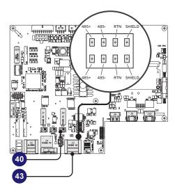
For long distance connections is necessary to use a shielded twisted pair cable with characteristic impedance of Z0=120 Ohm as shown on the following table:
