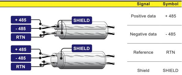
**NOTE** – Shield continuity must be provided along the communication line and must be grounded in a single point.
