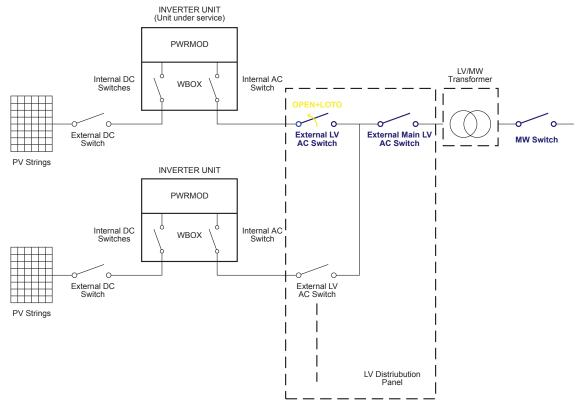
Open the external AC disconnect switch or the main external AC disconnect switch (blue in previous picture) outside the inverter (IEC 60364-7-712.536.2.2). In case none of the LV AC switches are present, the MV switch must be opened.
