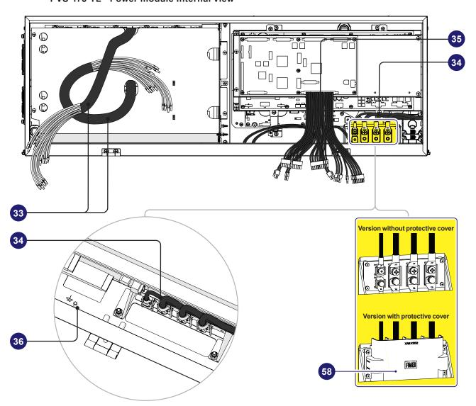
PVS-175-TL - Wiring box Internal view
