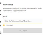
To access on the Web User Interface with the "Admin Plus" user privileges it's required to enter a security token that can be obtained by registering on the website <a href="www.fimer.com">www.fimer.com</a> (Refer to <a href="""">"""">""""" (Refer to make the website was and "Admin Plus token")</a> paragraph for further informations).
