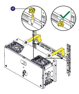
Remove handles (04) or other lifting device (if used)  Lift the power module (01) up to the bracket (03) and over the wiring box (02), using the handles (04) or the M8 eyebolts.
