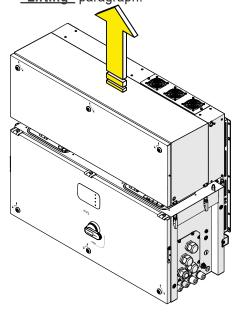
⚠ ATTENTION - Never leave the power module (01) or the wiring box (02) disassembled on the field. In case is necessary to disassemble the power module (01) only, a IP65 protection covers for wiring box openings (for temporary installation of wiring box only) kit is available as accessory options.
