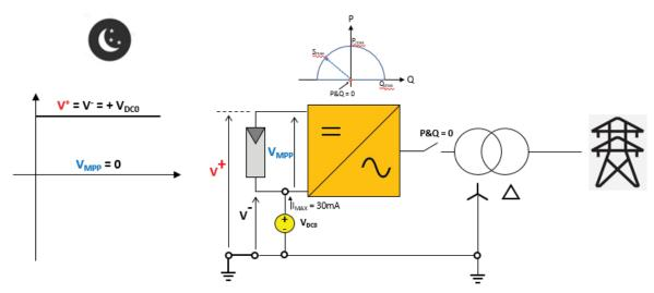
In the figure PVS-175's array terminal voltages with respect to ground during night-time operation of the Anti-PID board, inverter is off-line
