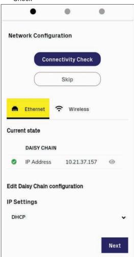
MOTE – When the networking configuration is concluded, it is possibile test the inverter connectivity to internet and Aurora Vision cloud services.
