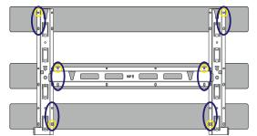
Frame mounting (3 supports) minimum fixing points
