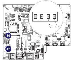
**NOTE** – In case of the DRM0 function is activated without the proper wiring of the Remote terminal block **(42)**, the inverter will no longer be able to connect to the grid. For further information regarding the DRM0 function refer to the AS/NZS 4777 standard.
