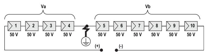
Va = voltage measured between + pole and = 200V
