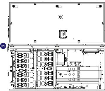
The layout of the DC surge arrester boards (21) is provided below, with reference of the points where the input DC voltage absence test must be performed. The points are represented by the faston where the cables (coming from DC switches (19)) are connected.
