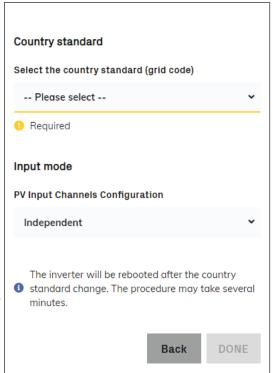
NOTE – After the grid standard is set you have 24 hours to make any changes to the grid standard value; 24 hours later the Country Standard will be locked. In case of subsequent needs of change of grid standard, the remaining time shall be reset in order to have the 24 hours of unlocked operation available again (refer to "USER menu" and "SERVICE TOOLS menu" sections of Web UI to know how to unlock the Country Standard).
