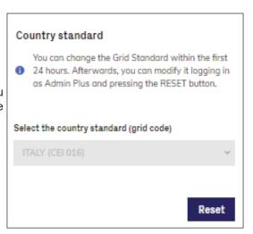
NOTE – After the grid standard is set you have 24 hours to make any changes to the grid standard value; 24 hours later the Country Standard sub-menu will be locked, and any subsequent changes might only be made accessing with Admin Plus privileges. Refer to the dedicated section on "USER menu" and "SERVICE TOOLS menu" to know how to unlock the Country Standard sub-menu.
