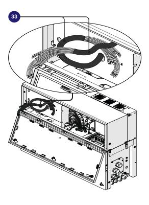
Wrap the DC interface cables (33) with the two cable sheaths supplied in the wiring box installation kit.
