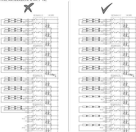
Ns < 12 (11 in this example): connect one string each from MPP1 to MPP11 or from MPP2 to MPP12.
