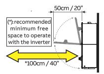
Do not install any object (e.g. AC or DC cables) that could be damaged by overheating from outgoing
