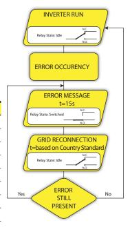
In the presence of W003, W004, W005, W006, W007 signalling, the alarm contact switches and then reset itself at the end of the alarm signal. This means that during the absence of grid voltage (display message "Missing Grid") the alarm contact remains in its resting position.
