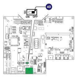
**NOTE** – Each inverter is shipped with the RS485 address pre-set to "2" and with the resistance terminal setting Switch (40) in the OFF position.
