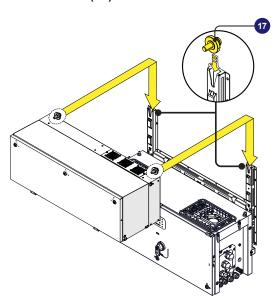
ATTENTION – During this installation phase pay special attention to not damage the gaskets on the AC and DC coupling system.
