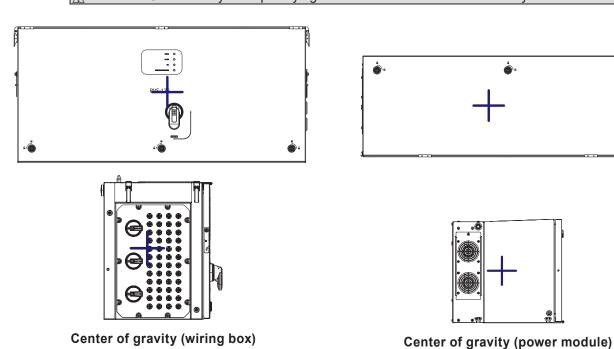
⚠ ATTENTION - In case of manual lifting it's suggested to use a support plan (e.g. a table) to place the equipment during the lifiting operation, in order to allow the change of hands position.
