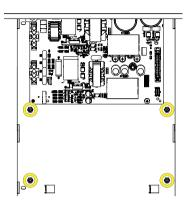
•Install the pre-charge board (01) on the 4 standoffs and lock it using the four M4 screws (supplied in the kit).
