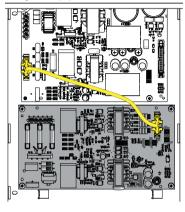
• Connect the AC grid voltage wiring :
