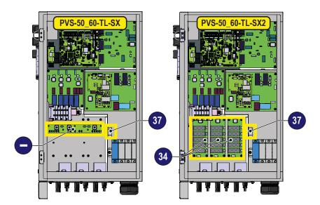
In case of absence of voltage between "Positive-earth" and "Negative-earth" check that there is no voltage on the all DC branches coming from the photovoltaic field, measuring between all the points:
