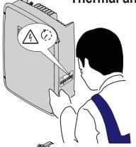
WARNING: the removal of guards or covers is only permitted after the voltage has been removed and time period indicated on the label has passed. This is to let the components cool down and allow the internal capacitors to discharge. Refer to "Inverter switch-off" chapter on this manual to know all the necessary step to safely operate on the inverter.
