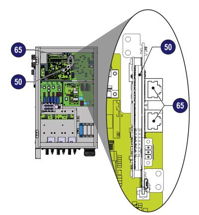
Connection of ethernet cable is made trought the two RJ45 connectors 65.
