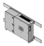
• The vertical installation is also permitted on a structure which must be composed of a support for the attachment of the bracket and one for the support of the rear pins.
