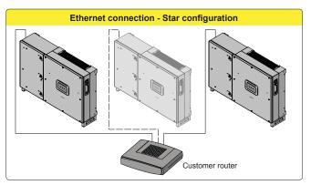
On each configuration of connection the maximum length of the cable must be 100m maximum between inverter – inverter and inverter – switch.
