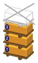
If the package is stored correctly, it can withstand a maximum load of 3 stacked devices (divided into 3 pallets).
