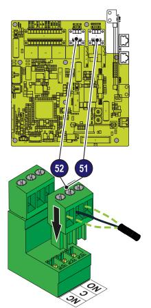
The inverter is equipped with 2 multifunction relays with configurable activation. It can be connected with normally open contact (being connected between the NO terminal and the common contact C) and with normally closed contact (being connected between the NC terminal and the common contact C).
