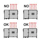
If the space available does not allow this arrangement, position the inverters in a staggered arrangement as shown in the figure so that heat dissipation is not affected by other inverters below.
