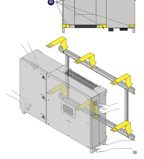
Install the 4 fixing braket on the 4 corner of the inverter (using 8 screws)
