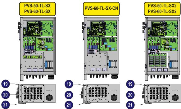
Refer to the document "String inverter – Product Manual appendix" available at www.fimer.com to know the brand and the model of the quick fit connector. Depending on the model of the connector of the own inverter, it is necessary to use the same model and the respective counterpart (check the compliant counterpart on the website of the manufacturer or in FIMER)
