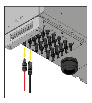
• Remove all quick fit DC connector (19 (20 (PV Connector)) from the wiring box. To avoid mechanical interferences, use a cable tie to collect the disconnected cables.
