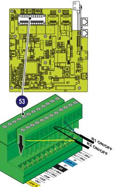
The connection and disconnection of the inverter to and from the grid can be controlled through an external control.
