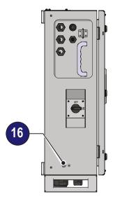
As alternative is possible to connect the earth cable to the protective earth terminal (external) <sup>16</sup> positioned on the left side of the mechanics. As per the protective earth terminal (internal) <sup>37</sup> following to the sequence illustrated in the below figure and tightening it to a torque of 11Nm. A ring cable lug, suitable for a M6 size threaded insert, must be installed on the cable.
