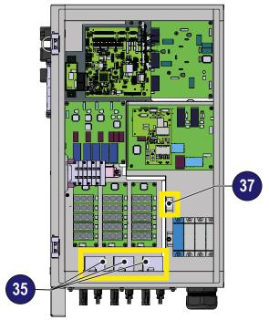
• Check the absence of voltage on the DC terminal block measuring between "Negative ( or 4 based on the product model) and protective earth terminal 7.
