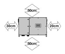
• Respect the minimum distances from objects around the inverter that could prevent the inverter installation and restrict or block the air flow.
