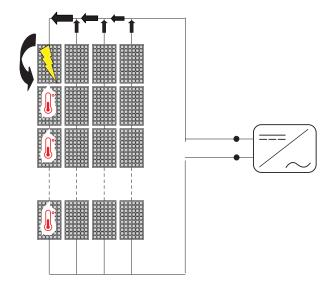
In these versions, you must directly connect the individual strings coming into the inverter (do not make field switchboards for parallel strings). This is because the positive side (+) 33 and negative side (-) 34 string fuses, situated on each input, are not rated to take strings in parallel (array). This operation can cause damage to the fuse and consequently malfunctioning of the inverter.
