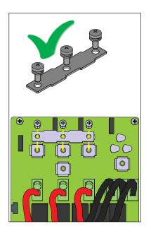
In the inverter -SX and -SX2 versions, the configuration of the input channels (MPPT) can be set in parallel. **Before carrying out this configuration, disconnect the strings from the inverter and open the AC disconnector.** This means that the parallel bar (supplied) must be installed on the parallel MPPT connection points 41, and that the software setting "parallel channel mode" should be performed on the inverter; this setting can be done by different way:
