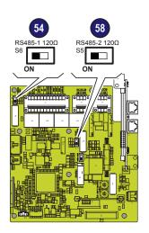
When connecting a single inverter to the monitoring system, activate the communication line resistance terminal by setting the switch 64 or 69 (to the ON position).
