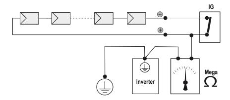
**MODELS - TL (without isolation transformer).** If the measured isolation resistance (Riso) is less than 500 MOhm, the inverter may not connect to the grid because of low isolation of the PV generator to ground.
