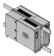
The vertical installation of two inverters positioned back to back is also permitted on a structure which must be composed of a support for the attachment of the brackets and one for the support of the rear pins.
