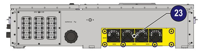
3. Pull out the cooling section
