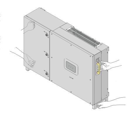
• Insert the heads of six anchor point 13 present on the bracket into the slots on the rear of the inverter.
