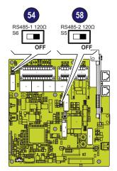
When an RS-485 connection is being used, if one or more inverters are added to the system at a later time, it is necessary to remember to reset to OFF the switch on the termination resistance being used (1) or (2) on the inverter which previously was the last in the system.
