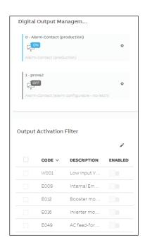
This section of the menu allows you to set the activation status of a relay (available either as contact normally open - N.O. - and as a normally closed contact -N.C.) and to configure customised alarm conditions.
