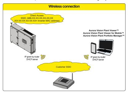
During the installation wizard of the single inverter, the installer will be asked to connect the inverter to a Wi-Fi router. By selecting connection to Wi-Fi router the inverter will turn on a second Wi-Fi radio channel in order to enable connection to the Wi-Fi router. By selecting "Skip this step" button the other radio channel will be kept off.
