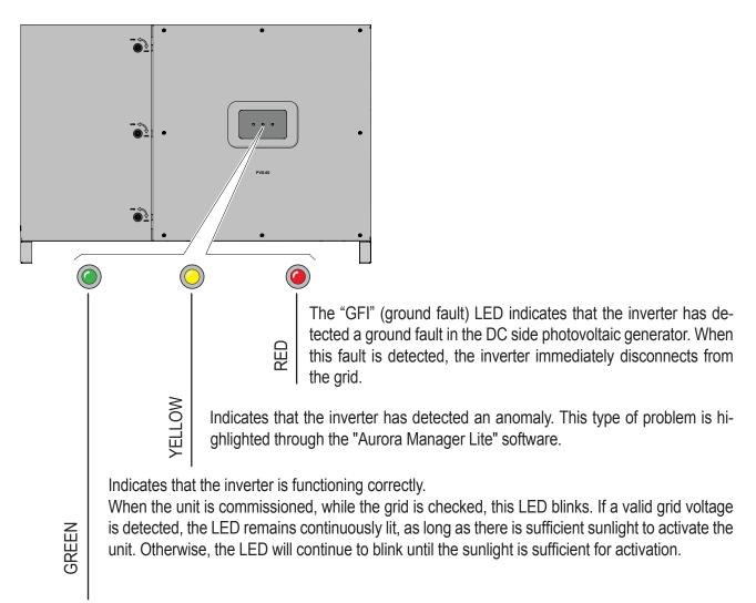
The LEDs, in various multiple available combinations, can signal multiple conditions other than the original single condition; see the various descriptions explained in the manual.
