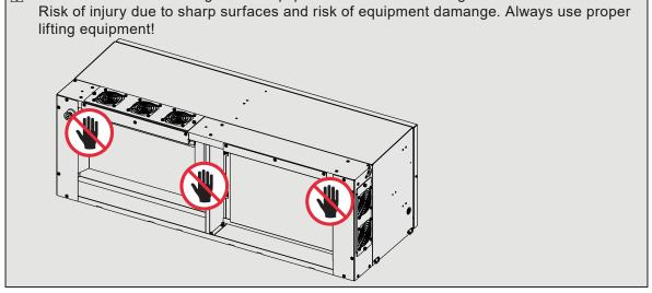
It is required to use one of the following lifting methods to move the equipment during installation or maintenance phases:
