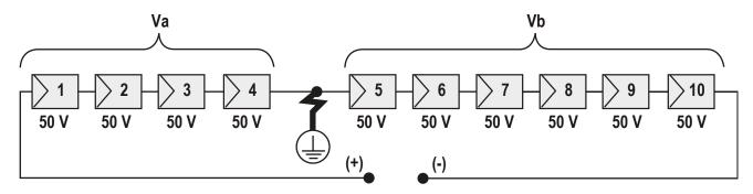
Va = voltage measured between + pole and  $\bigoplus$  = 200V Vb = voltage measured between - pole and  $\bigoplus$  = 300V In all measurements with  $\bigoplus$ , the ground of the inverter is indicated.
