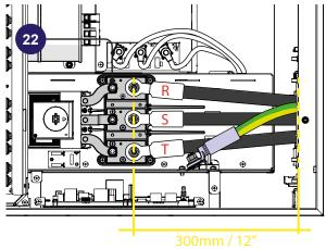
▲ ATTENTION – In case of a wrong phase sequence the inverter will not connect to the grid and it will provide an error state.
