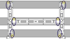
Frame mounting (2 supports) minimum fixing points
