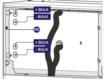
• The layout of the DC input filter board is provided below, with reference of the points where the input DC voltage absence test must be performed.
