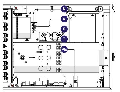
14. Voltage absence test on bulk capacitors (Power Module)
