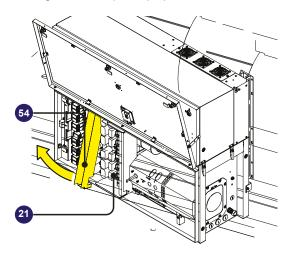
• Remove the three M5 screws from the DC surge arrester plate.
