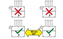
• The installation of two inverters positioned back to back is also permitted on a structure which must be composed of 2 or 3 frame supports (refer to "Mounting with a support bracket" chapter). In this case the minimum recommended distance between the units in order to avoid the use of an air deflector is 30cm.
