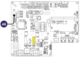
Procedure to replace the RS485 line communication board (46):
