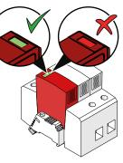
Procedure for replacing one of the AC surge arrester cartridges (23):
