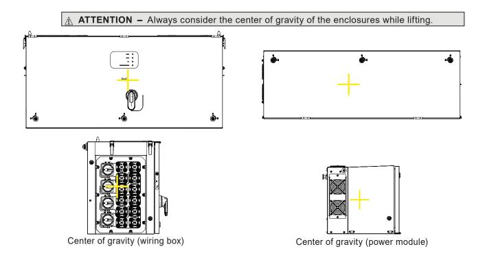
▲ **ATTENTION** – In case of manual lifting it's suggested to use a support plan (e.g. a table) to place the equipment during the lifting operation, to allow the change of hands position.
