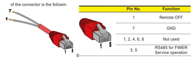
• Connect the modified RJ45 cable to the external RJ45 connector (56) to perform a soft shut-down of the inverter. The connection of the cable will causes the interruption of the operation of the inverter, i.e. it stops the IGBT switching, interrupts the injection of current into the grid and open the AC contactor.
