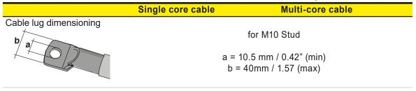
▲ **ATTENTION** – The AC connection busbars (22) are in copper tin-plated; therefore if aluminum cables are used, the correct coupling with the copper bars must be guaranteed by using appropriate bi-metallic cable lug.
