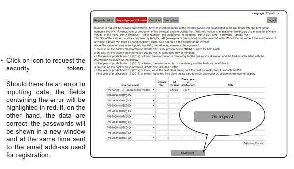
A ATTENTION - The security token enables the "Admin Plus" privileges which allows the inverter's sensitive parameters to be changed. Proceed to changing the aforementioned parameters only when requested by the grid operator or by customer assistance.
