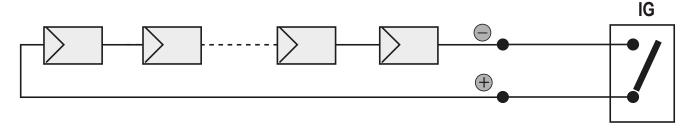
Once the short-circuit has been made, measure the isolation resistance (Riso) using a megohmmeter positioned between the two shorted poles and ground (of the inverter).
