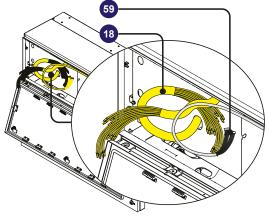
• Wrap the DC interface cables (18) with the two cable sheaths supplied in the wiring box installation kit.
