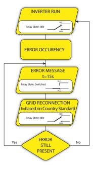
In the presence of W003, W004, W005, W006, W007 signalling, the alarm contact switches to then reset itself at the end of the alarm signal. This means that during the absence of grid voltage (display message "Missing Grid") the alarm contact remains in its resting position.
