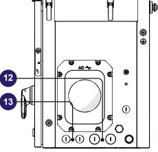
NOTE – Use UL Listed reduction washers in case of smaller conduit used to maintain Type 4 enclosure integrity.
