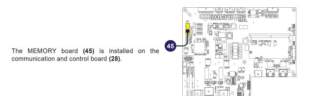
Procedure to replace the MEMORY board (45):
