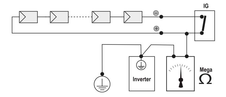
If the measured isolation resistance (Riso) is less than 33 kOhm, the inverter may not connect to the grid because of low isolation of the PV generator to ground.
