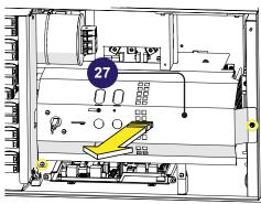
• Pass the protective earth cable through the AC opening (size 3" conduit) (11) on the AC panel.
