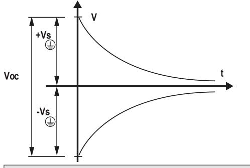
NOTE – The internal resistance of the voltmeter tends to zero the voltage present on the PV generator due to the capacitive effect.
