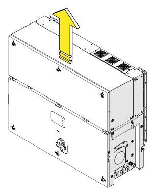
• Remove the power module **(01)** following the indications for the mounting procedure in the "Mounting with a support bracket - Assembly the Inverter to the bracket" chapter in the reverse order and the indication for lifting methods in "Type of lifting" chapter.
