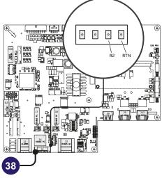
The external switch used for Remote ON/OFF should be rated for DC low voltage, low current application (the minimum switching current capability should be 1mA or lower).
