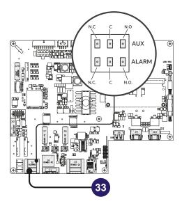
Different types of devices (light, sound, etc.) can be connected to the relay, provided they comply with the following requirements:
