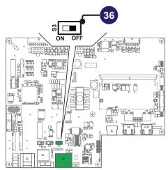
When an RS-485 connection is being used, if one or more inverters are added to the system at a later time, it is necessary to remember to reset to OFF the switch of the termination resistance being used (1) or (2) on the inverter which previously was the last in the system.
