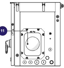
ATTENTION – Use UL Listed reduction washers in case of smaller conduit used to maintain Type 4 enclosure integrity.
