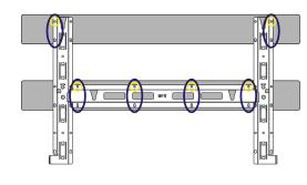
NOTE – In case of use of "frame fixing brackets" (see picture as example) it will be possible to fix the bracket to the frame structure without drilling any additional holes.
