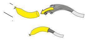
• Remove the cable tie from the AFD interface cables (59) and pass them into the wiring box using the dedicated opening for interface cables.
