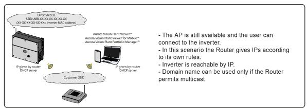
During the installation wizard of the single inverter, the installer will be asked to connect the inverter to a Wi-Fi router. By selecting connection to Wi-Fi router the inverter will turn on a second Wi-Fi radio channel in order to enable connection to the Wi-Fi router. By selecting "Skip this step" button the other radio channel will be kept off.
