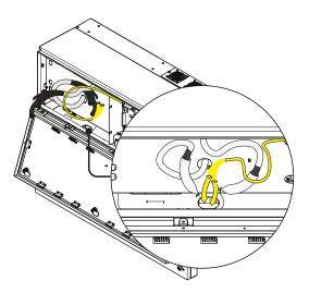
• Pass the DC interface cables (18) into the same dedicated opening used for the AFD interface cables.
