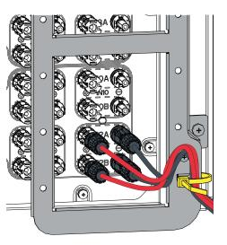
• Follow the installation order shown in the figure, to connect the cables neatly. The figure also indicates the right holes on the cable tray that must be used to block the cables of each MPPT.
