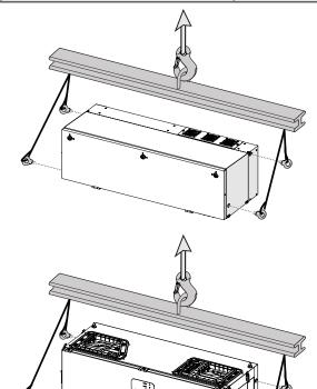
M8. Hole for Eyebolts UNI2947 (not supplied) \*lifting balancer must be 20 cm longer (per side) than the lifted device.
