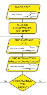
If the alarm condition is persistent, the relay will remain activated (status:switched)
