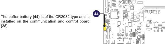
installed on the communication and control board (28).
