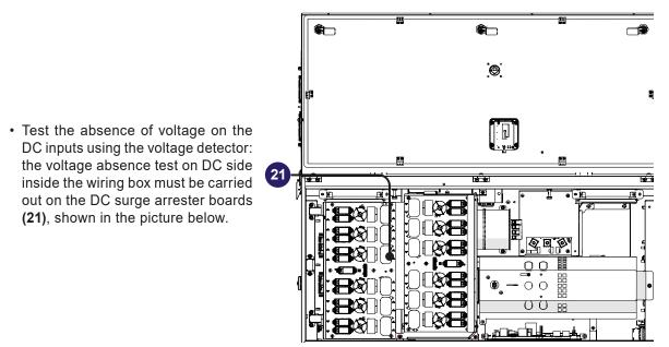
The layout of the DC surge arrester boards (21) is provided below, with reference of the points where the input DC voltage absence test must be performed. The points are represented by the faston where the cables (coming from DC switches (16)) are connected.
