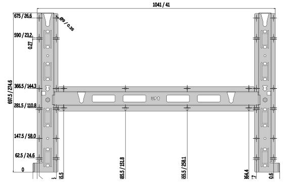
The diameter of holes in the bracket are 9mm / 0,35".
