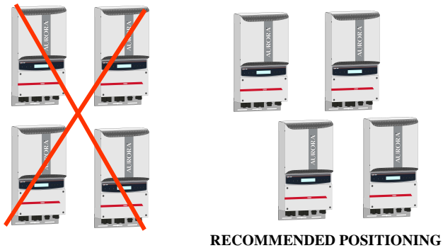
Fig. 5 - Recommended installation of AURORA inverters
